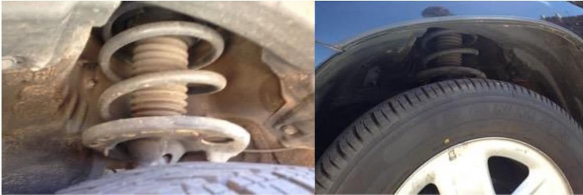
**Figure 1.2-4: Helical Coil Compression Spring behind the wheel, a – close up and b – distant view**
