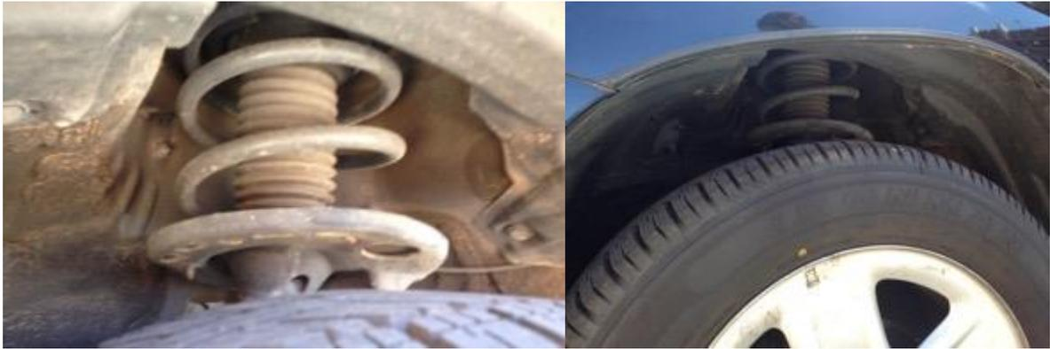
Figure 1.3-2: Helical Coil Compression Spring behind the wheel, a – close up and b – distant view
