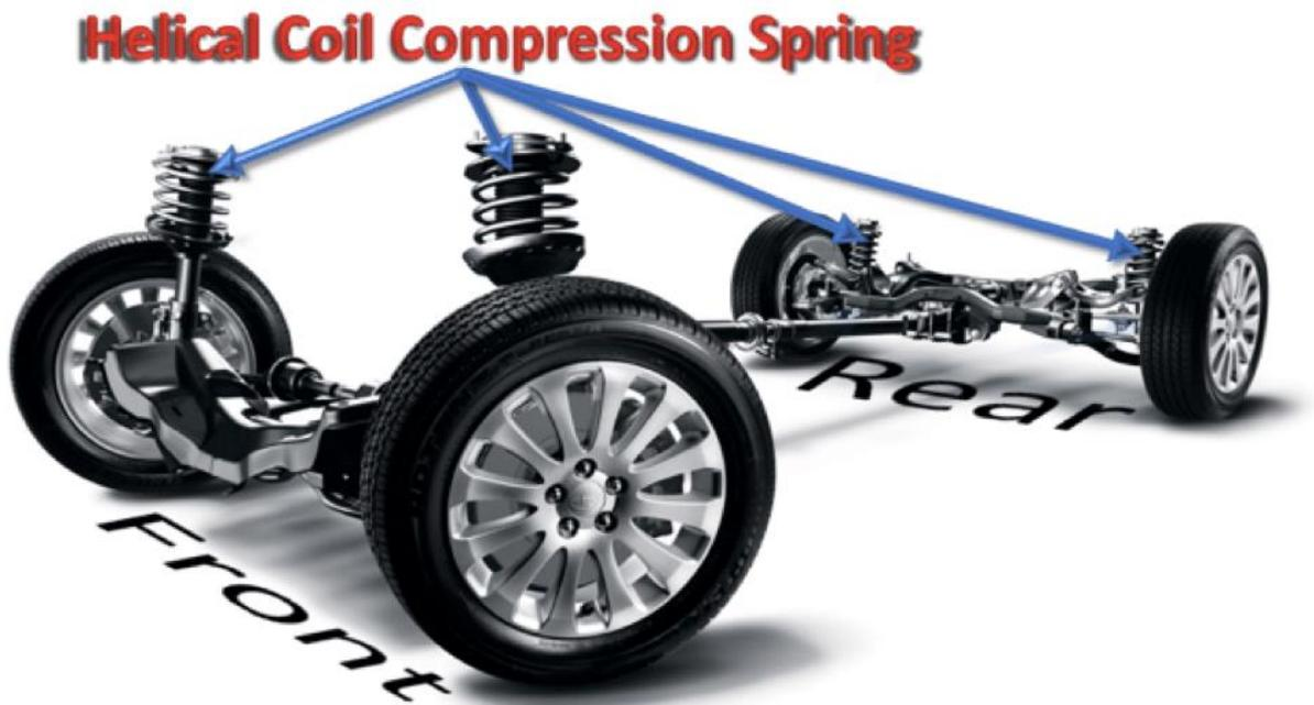
Figure 1.2-3: Four Springs in the chassis design
