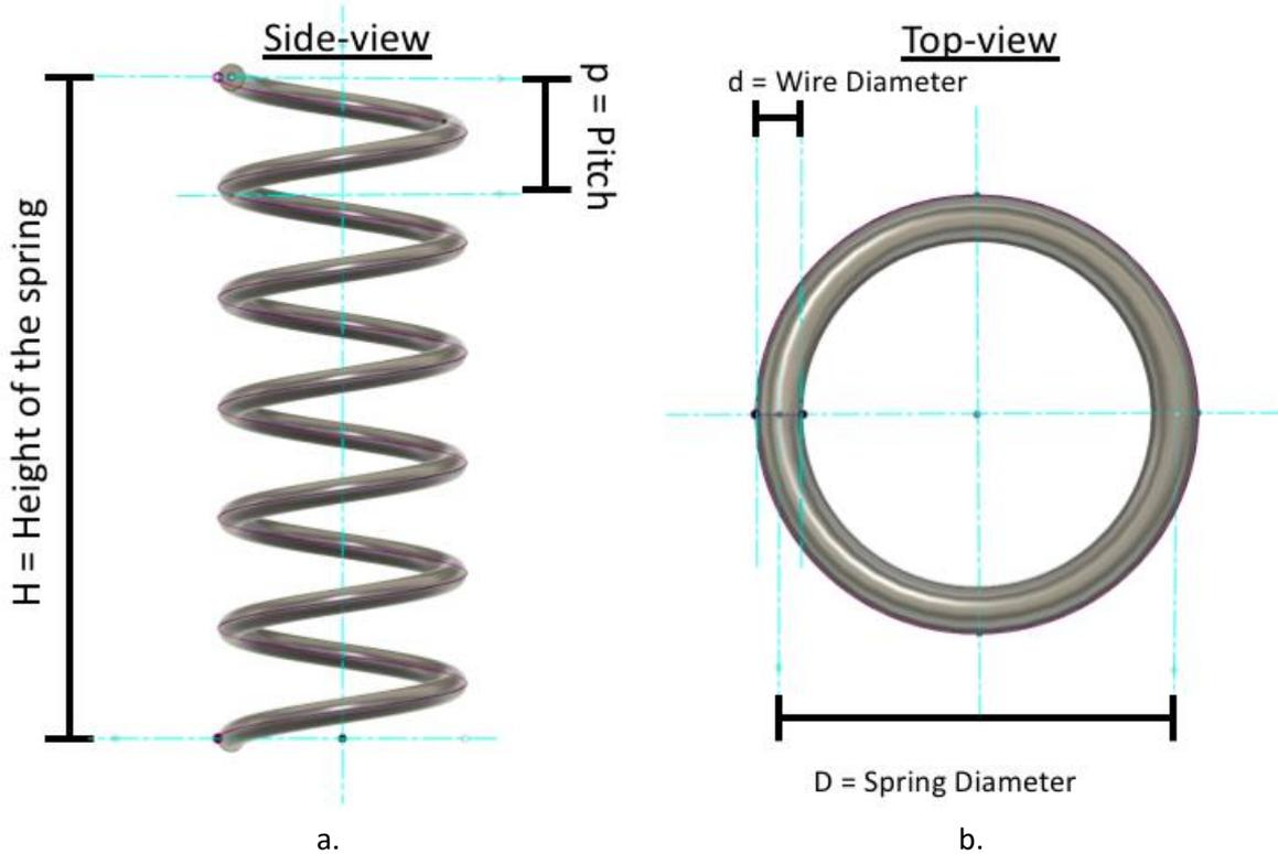
Figure 2.1-2: Side and Top of view of the spring
