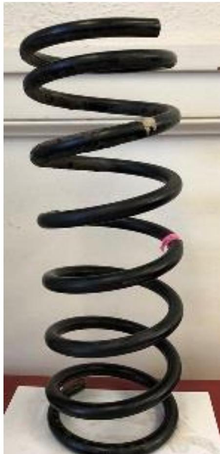
Figure 2.1-1: Helical Coil Compression Spring
