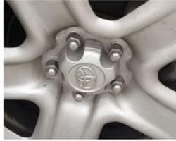
**Figure 2.1-3: Hub of the front right wheel where the lug stud goes**
