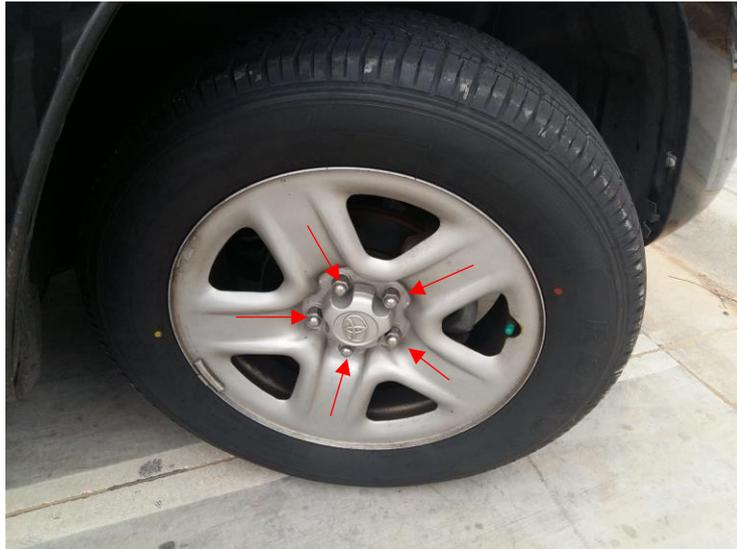
**Figure 2.1-5: Location of lug stud on the front right wheel**
