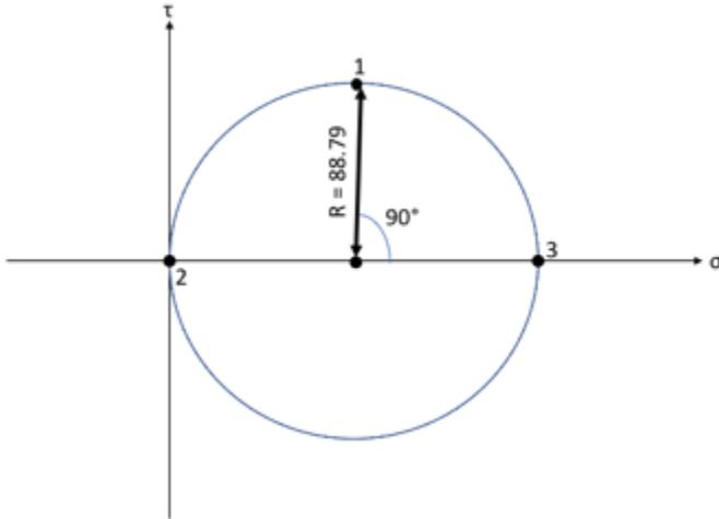
Figure 3.3-2: Mohr's Circle for lug stud before loading
