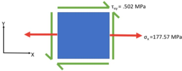
Figure 3.3-1: Stress element before loading
