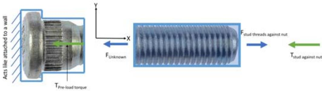
**Figure 1-4: Free body diagram of a lug stud**
