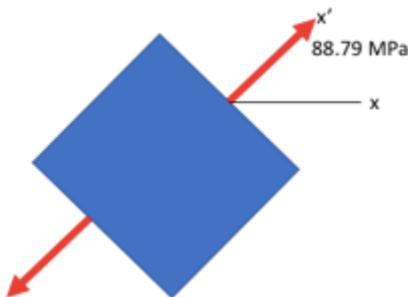
Figure 3.3-3: Stress element after orientation
