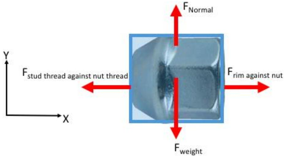
**Figure 3.2-1: Forces on a lug nut before loading**
