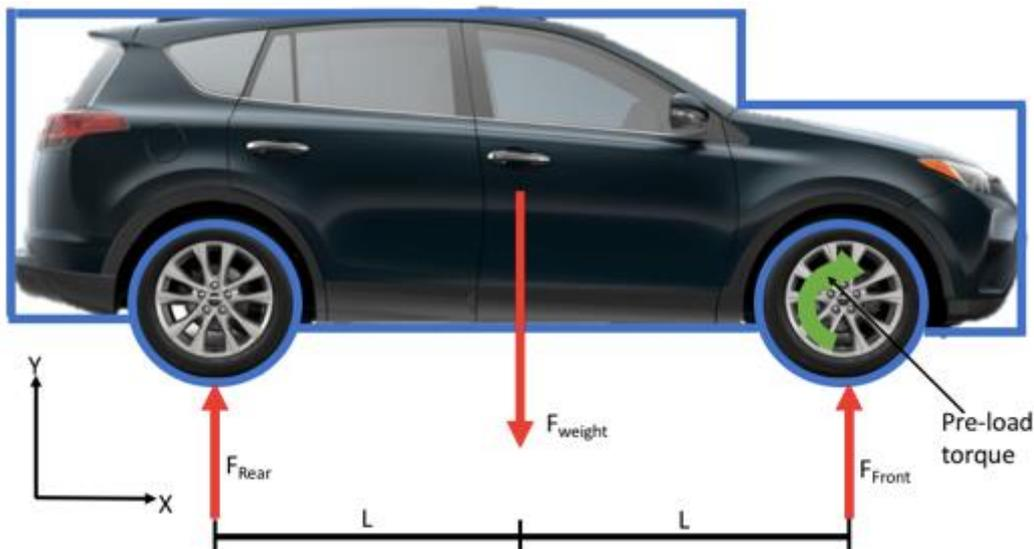
**Figure 3.1-2: Free-body diagram of RAV4 with reactions and pre-load Torque applied**
