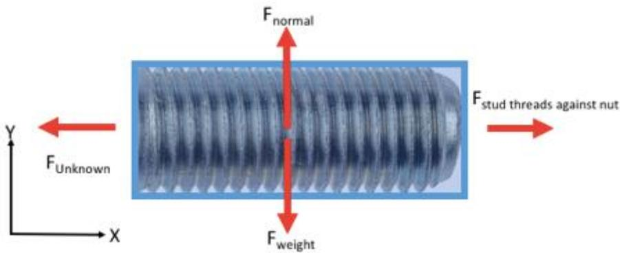
**Figure 3.2-3: Forces on a lug stud before loading**
