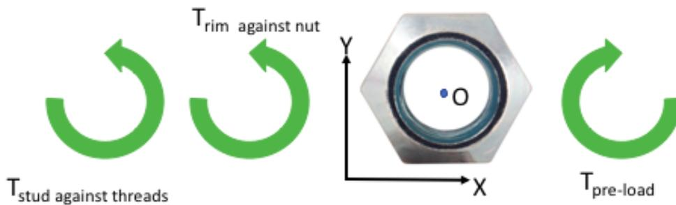
**Figure 3.2-2: Moments on a lug nut before loading**
