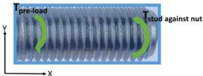
**Figure 3.2-4: Moments on a lug stud before loading**
