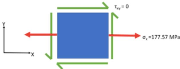
**Figure 3.3-4: Stress element after pre-loading**
