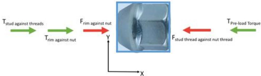
**Figure 3.1-3: Free Body diagram of a lug nut**
