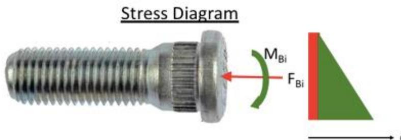
**Figure 5: Stress diagram of lug stud due to axial force and bending moment**
