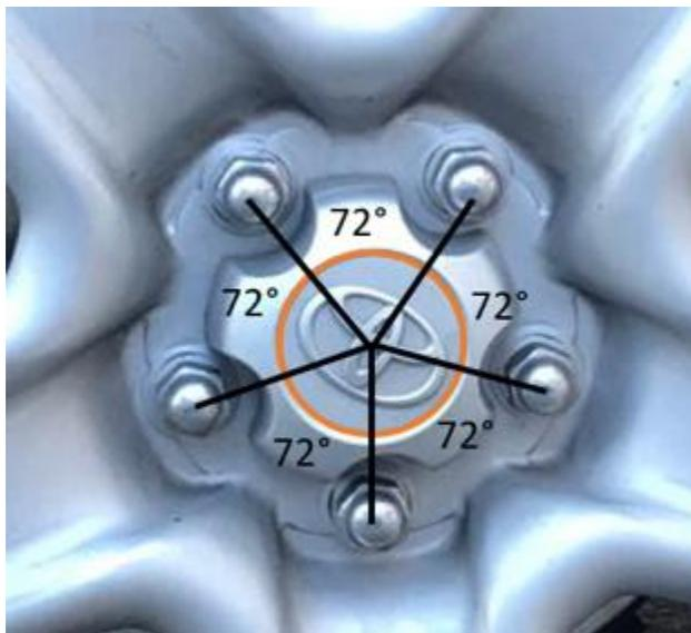
**Figure 4.1-3: Arrangement of lug studs in a pentagonal fashion**
