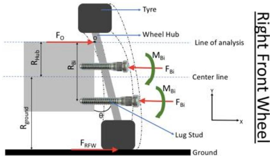
**Figure 4.1-2: Free body diagram of the right front wheel**
