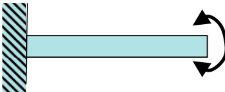
**Figure 5.2-5: Reversed Torsional Loading**
